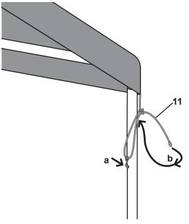
Figure 8: Securing Tarp Corner Hook (11)
